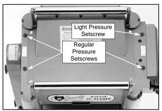
Figure 25. Roller pressure adjustment.
